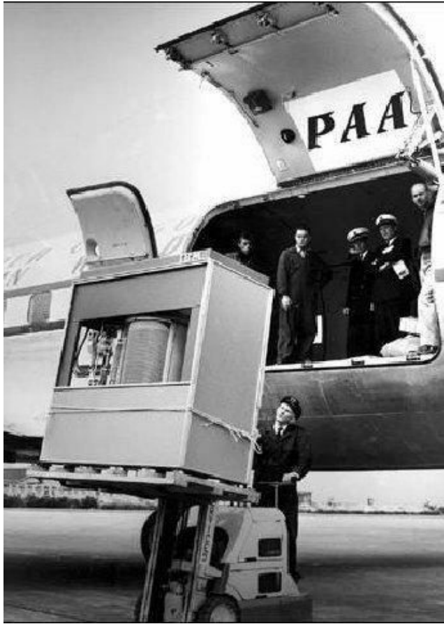
Figure 1: The picture aside shows the 350 Disk Storage Unit which consists the magnetic disk memory unit with its access mechanism, the electronic and pneumatic controls for the access mechanism, and a small air compressor. Assembled with covers, the 350 was 60 inches long, 68 inches high and 29 inches deep. It was configured with 50 magnetic disks containing 50,000 sectors, each of which help 100 alphanumeric characters, for a capacity of 5 million characters. Disks rotated at 1200 rpm, tracks (20 to the inch) were recorded at up to 100 bits per inch, and typical head to disk spacing was 800 micro-inches. The execution of a "seek" instruction positioned a read-write head to the track that contained the desired sector and selected the sector for a later read or write operation. Seek time averaged about 600 milliseconds. [Source: EETimes, and most of it was copied verbatim]
